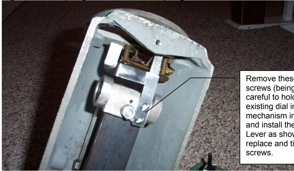
Fig 4 Attach Spring Lever to Rimac Spring
