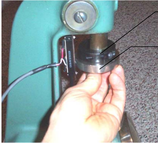
Figure 10 Reinstall Top Arbor Platform and Set Safety Stops
